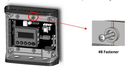
If the meter is not available for use as a drill template, a drawing indicating the spacing between mounting holes can be found in the appendix. The centerline holes are intended for fastening to wall studs. If hollow wall fasteners are used, the outer 4 mounting points are recommended.
