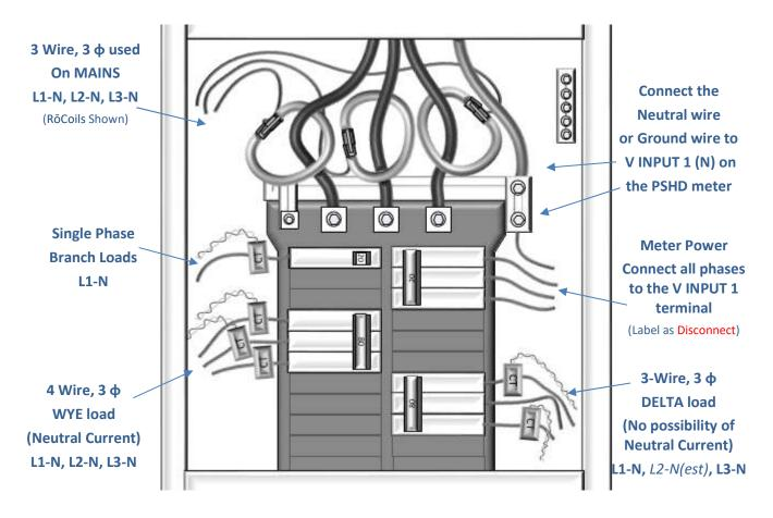
Illustrating the intended wiring configuration for each of the Service Types available in the Service drop-down list under "Meter Setup"
